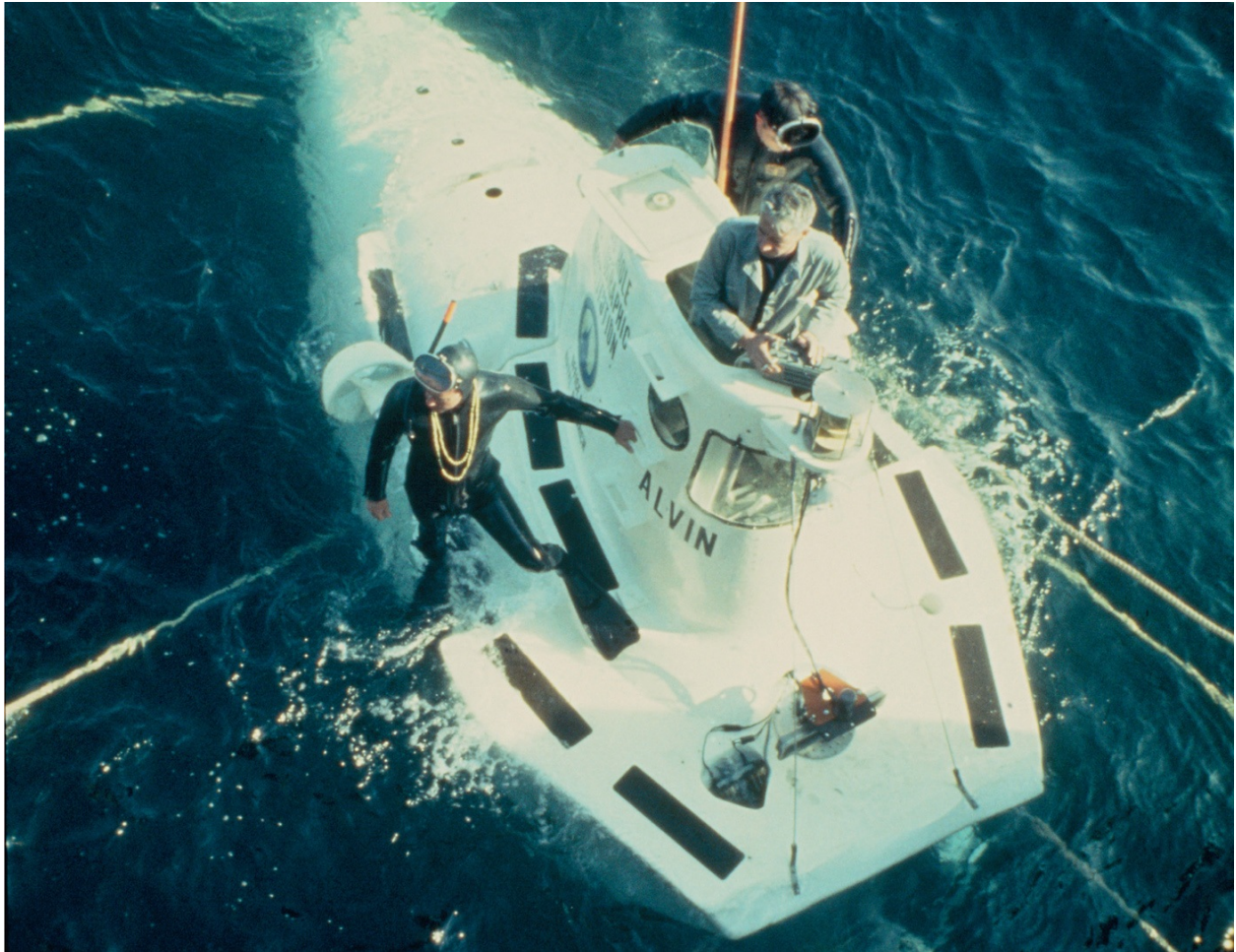
DSV Alvin , a manned deep-ocean research submersible, prepares to dive. The purpose of its mission was to explore the Atlantis Massif, a prominent mountain range deep below the surface of the Atlantic Ocean.
